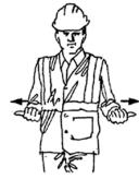
**Extend Hydraulic Boom**Both fists in front of body with thumbs pointing outward.
